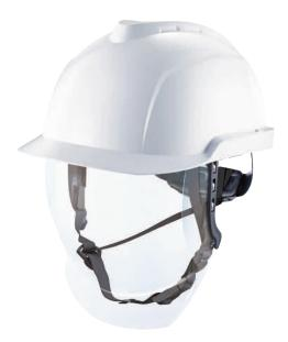
Balanced lightweight electrician's safety helmet, non-vented, with 6-point Fas-Trac<sup>®</sup> III ratchet suspension and GS-ET-29 class 1 face shield certified for protection against arc flash. For use where top impact hazards to the head, chemical splash, Ultra-Violet radiation, molten metal splash or electric arc to the face exist.
